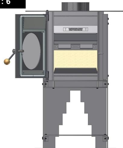
Once the vermiculite board back is in place, ensure jet inlet holes on the back plate are clear of any obstructions.
