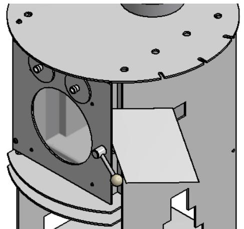
Nip up screws while holding door in place, then tighten fully with a 5mm Allen Key.
