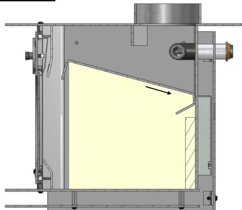
Push the baffle right to the back of firebox.
