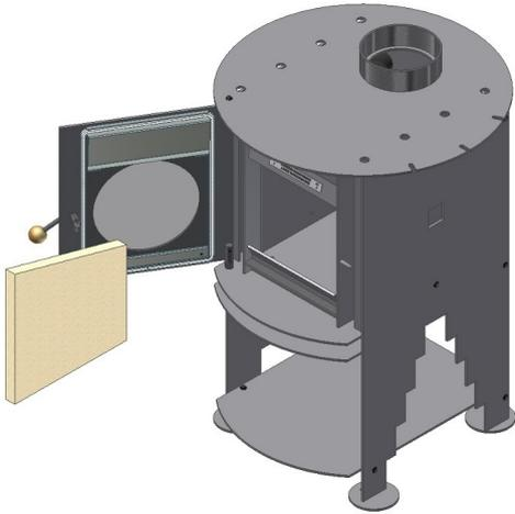
Place one Vermiculite board side brick into the Firebox as shown above.
