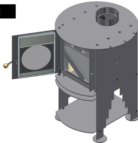
Put the steel baffle in on an angle through the door frame. Lift it up holding it horizontally resting on the one side bricks.
