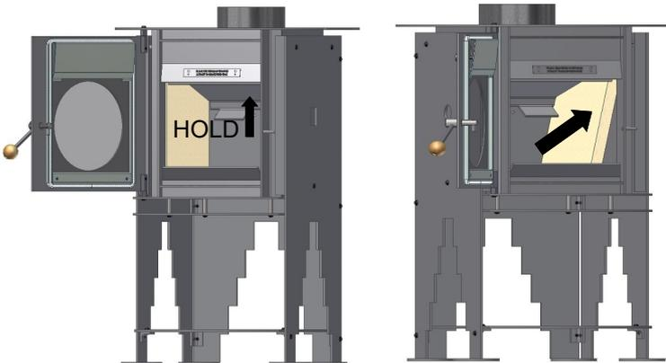
While holding up the steel baffle horizontally, insert the opposite side brick in from underneath it, as shown above. The 2 side bricks will now support the steel baffle.
