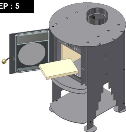
Fit back vermiculite board panel into the firebox back, ensuring that it is sitting hard against the back of the firebox.
