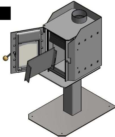
Put the steel baffle in on an angle through the door frame.
