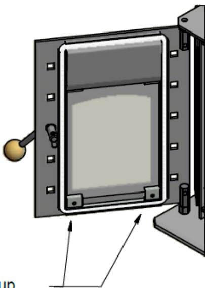
Slide Glass up & screw bottom Glass Retainers on
