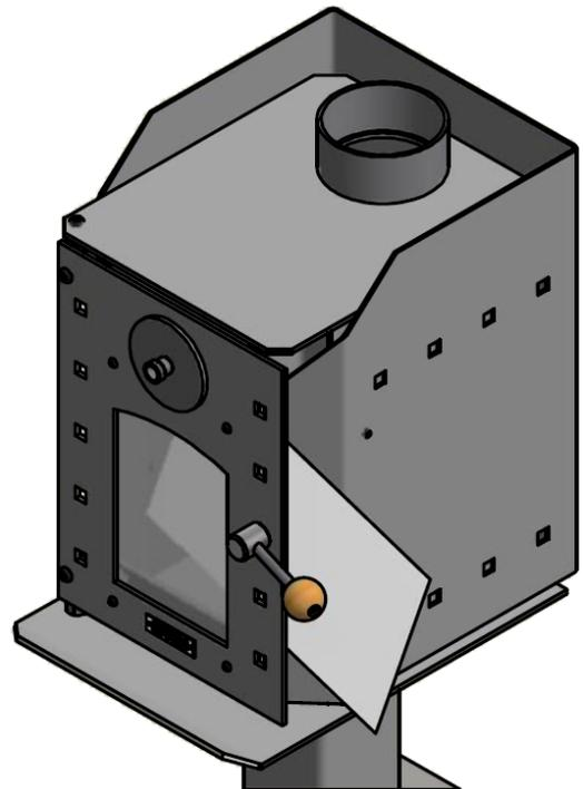
Nip up screws while holding door in place, then tighten fully with a 5mm allen Key.
