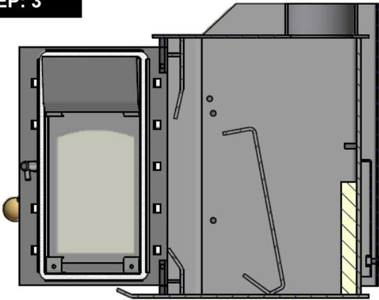
Straighten the steel baffle horizontally,
