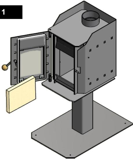
Place vermiculite board back brick into the back of the Firebox.
