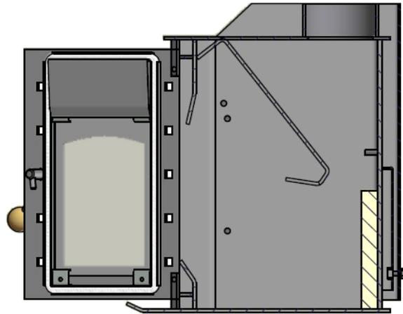
Push the baffle up to the top of firebox.
