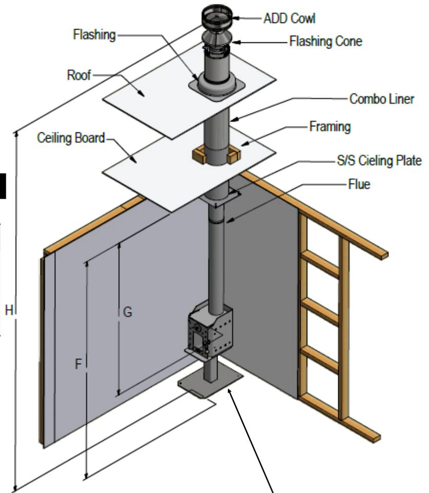
NOTE: Base of Pedestal option does not satisfy requirements for hearth when installed on combustible surfaces.
