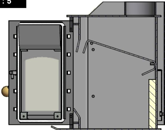
Push the baffle back so it rests on the support pins on the sides and the firebox back.
